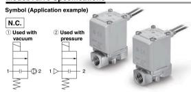
When the valve is closed, flow is blocked from port 1 to port 2. However, if the pressure in port 2 is higher than port 1, the valve will not be able to block the fluid and it will flow from port 2 to port 1.
